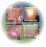
Unlike silicon-based solar cells, dyesensitized solar cells offer transparency, low cost, and high power-conversion efficiencies under cloudy and artificial light conditions.
