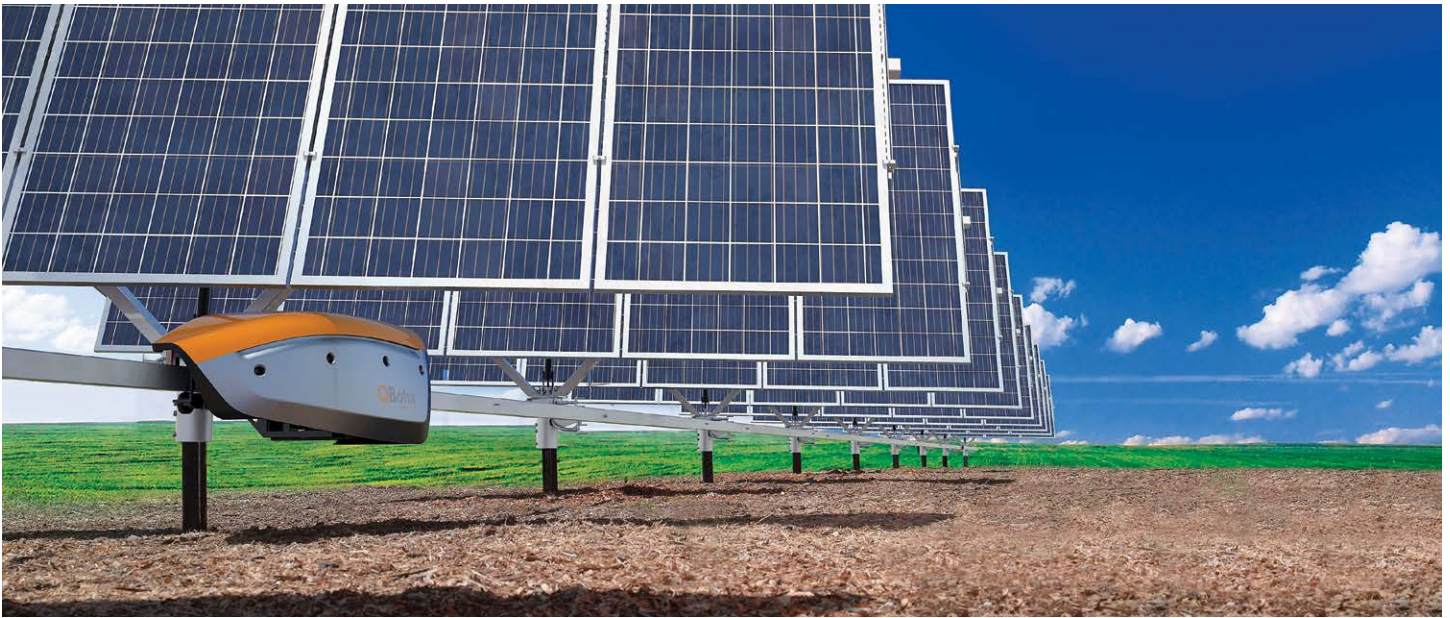
Figure 2. Incubator awardee QBotix has developed a robotic tracking system that increases solar PV power plant production by up to 45% and delivers cost savings up to 20%.
