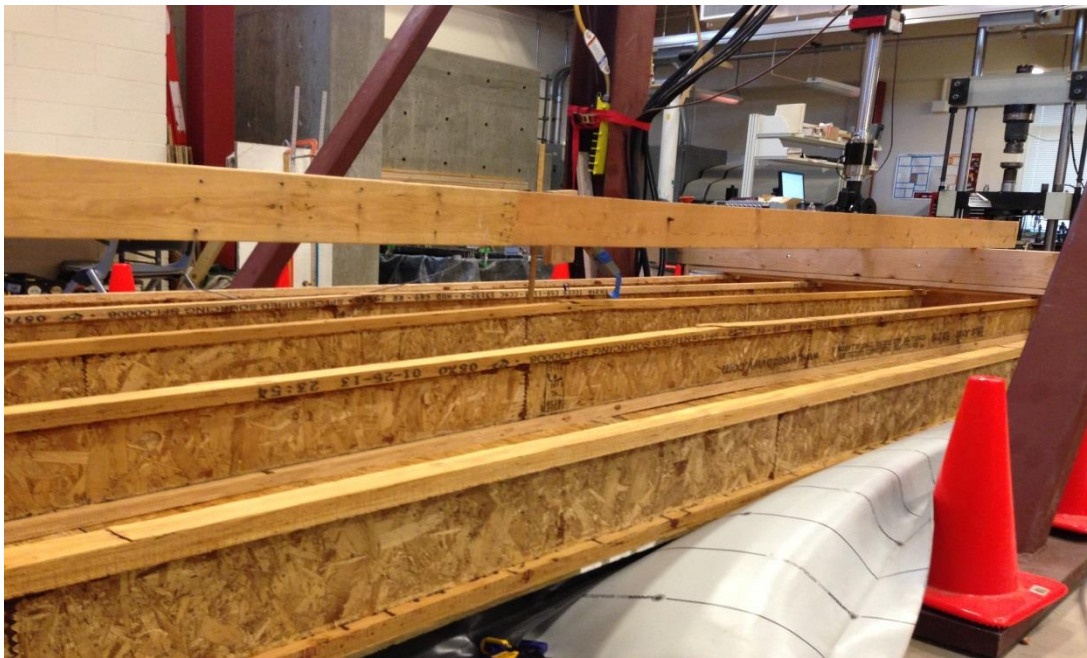
Figure 29. Failure in TJI roof test assembly.
