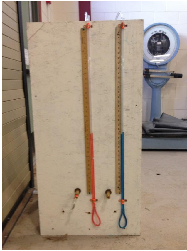
Figure 20. Photograph of double manometer use in laboratory.
