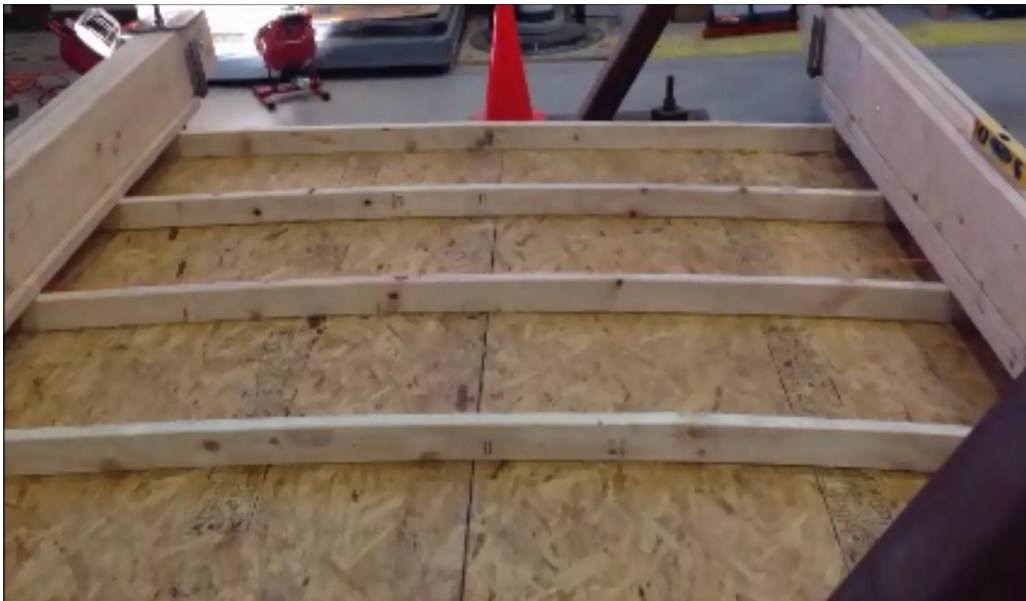
Figure 15. Photograph of roof assembly under load.
