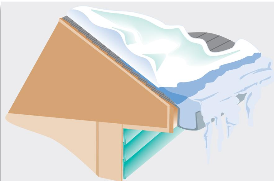
35-psf snow load according to current code. The first case represents a snow load condition immediately following a snowfall. For this case, a uniform 35-psf snow load was applied to the collector and to the rafter outside of the collector footprint. The snow load on the collector was translated to point loads on the rafter at the rail locations.
