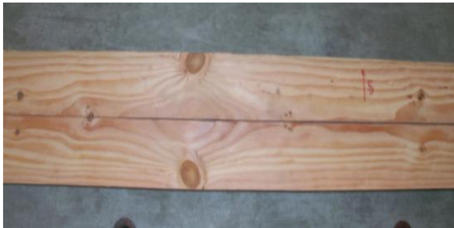
Figure 8. Twin 2" x 4" joists cut from a single 4" x 4" joist.
