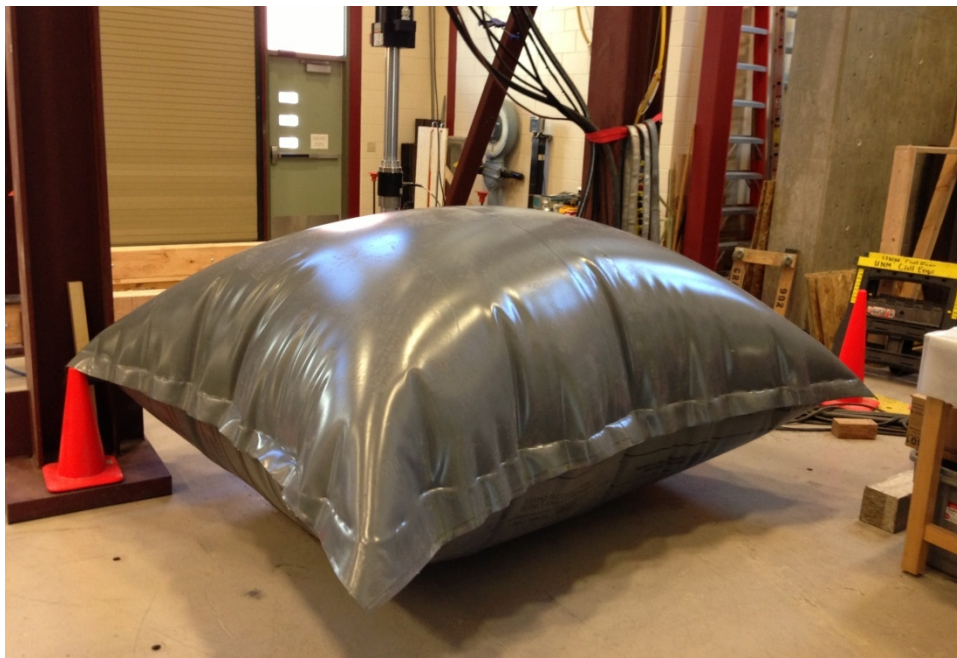
Figure 17. Photograph of 8' x 10' PVC air bladder.
