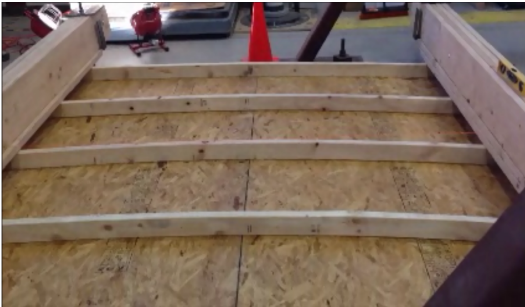
Figure 15. Photograph of roof assembly under load.
