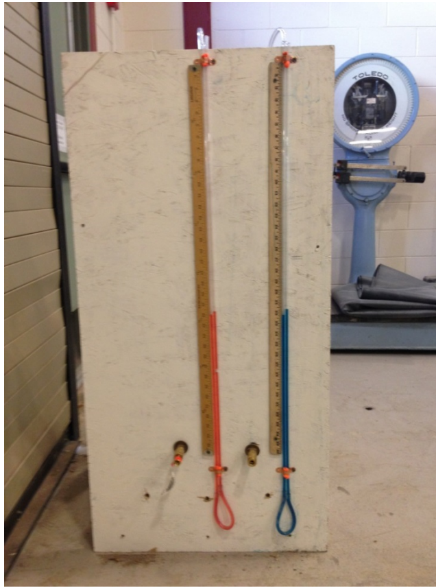
Figure 20. Photograph of double manometer use in laboratory.
