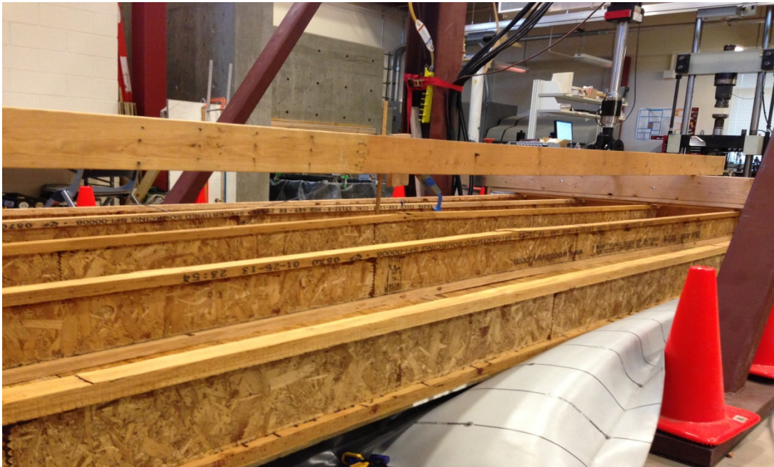
Figure 29. Failure in TJI roof test assembly.
