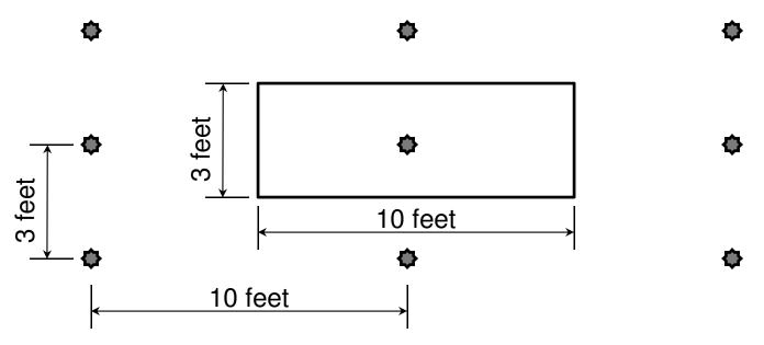
ASCE 7-05 section 4.3 "Unless otherwise specified, the indicated concentration shall be assumed to be uniformly distributed over an area 2.5 ft square and shall be located so as to produce the maximum load effects in structural members."
