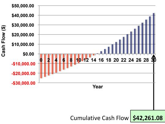
The calculated cumulative cash flow is equal to the height of the last bar on the PV System Cumulative Cash Flow chart.
